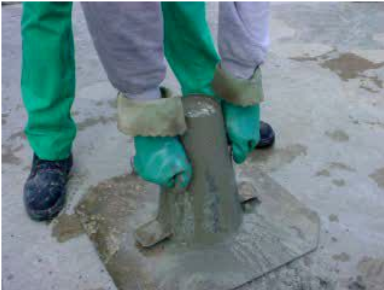
ABATIMENTO – SLUMP TEST 200 \pm 30 mm
